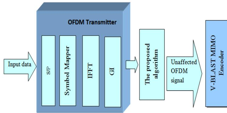
Fig. 4. SNFRbot MIMO-OFDM enhanced block diagram
