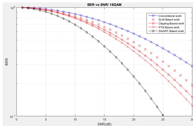
Fig. 7. BER curves based 16-QAM compared to literature
