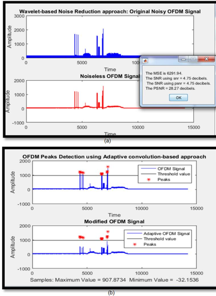
Fig. 2. a) Noise removal using SAT-based work, b) Odd peaks detected using SAT-based work [13]
